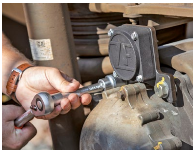
The ZF sensors are located on the bogie of the test train.
